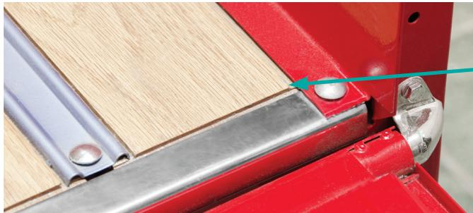
Bed wood goes over flange of front panel, under flange of bed sides.
