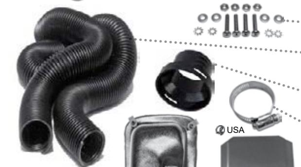
Defrost tube attaching hardware
