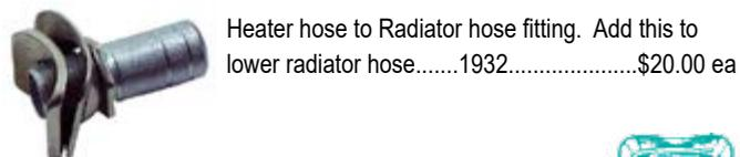
Heater hose to Radiator hose fitting. Add this to lower radiator hose.....1932..... \$20.00 ea
