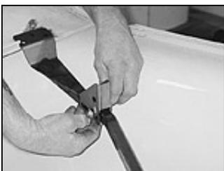
Now the top hinge brackets were bolted to each of the supports with the supplied hardware. These four oblonged holes are what give you your hood adjustment up front.
