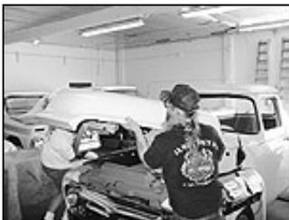
The hood was lifted off the truck and flipped over onto something soft so it could be worked on. The hinges were then removed from the cowl.
