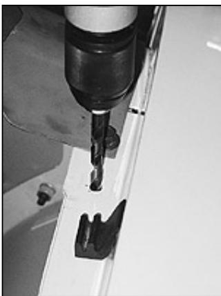
All that was left to be installed was the polished stainless prop rod. A hole was measured out and drilled into the fender edge
