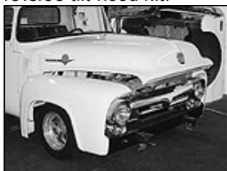
With the CPP kit, the hood slides up and out slightly to clear the fenders before it hinges forward.
