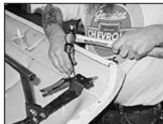
Alan used a small pair of Vise Grips to hold the supports in place while he marked and drilled the three holes on each side. Here he dimpled the metal with a punch to keep the drill bit from walking on him.
