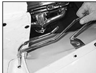
Two of the existing fender bolts were removed for the polished stainless track to be mounted. The rearmost bolt is what gives the rear of the hood its adjustment.
