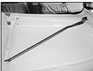
The new braces were then set in place and bolted to the rear of the hood.
