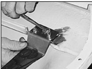
The supports were then bolted solid to the hood using the supplied hardware. Now the pivot bar could be removed.
