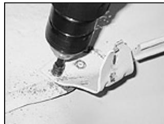
A special bit was used to cut out the three welds and remove the brackets. Then the area was ground smooth. If your truck is already painted, this is obviously an area you will need to be careful with.
