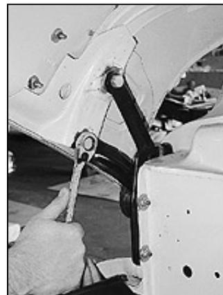
You'll need a friend's help right off the bat. The first step was to remove the four bolts that attach the hood to the hinges while supporting the hood.
