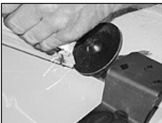
A die grinder was used to clearance a small portion of the metal lip so the supports would lay flush. This is another area where you'll need to take precautions to protect the existing paint.
