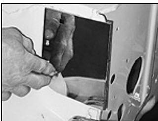
When you remove the stock hood hinges, you're left with four big ugly holes and maybe even some mismatched paint. The cool polished stainless covers were designed to eliminate a trip to the painter when you install the tilt kit. They simply slid on and were held with two carriage bolts.
