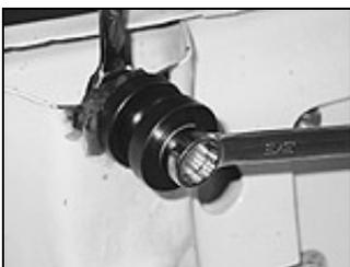
These Teflon rollers bolted to the existing hole in the bottom rear of each side of the hood.
