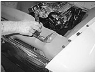
The lower hinges were bolted to the grille support using an existing hole. By installing the pivot bar (this time permanently and with a dab of grease), we could determine exactly where the second hole for the bracket needed to be drilled and bolted.
