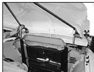
Now for the moment of truth. The hood was held in place while the pivot bar was inserted back into its brackets. Then the hood was carefully lowered into place and slowly closed. Now is the time to make all of the adjustments so the hood closes perfectly.
