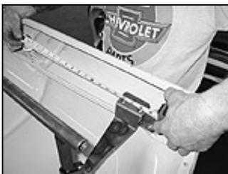
Using the tip of the hood spring as a reference point, the front brackets were measured out equally and marked.
