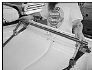
The pivot bar then temporarily dropped into the brackets so the supports could be aligned before being bolted to the front of the hood.
