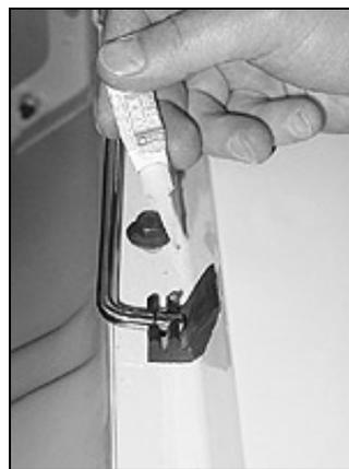
When the hood is closed, the rod rests in this modified factory fender rubber. It was simply glued into place.
