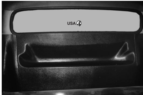
Shown is big back, covered, uncovered color is black. see how headliner is moulded to fit roof contour. Clips behind lip, easy, custom and clean install, no rubber retainer or clips
