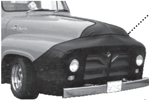
Bumper Mask is held on with bendable tabs
