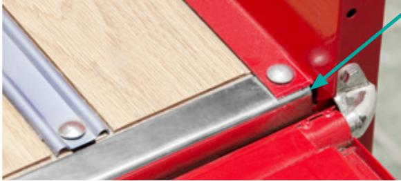
Note we do not indent ends of bed wood. We like the look better with end cap over bed flange instead of under, it is more level with strips and eliminates that dust catching crack. Grind down bed flange a tiny bit if you need to push the cap back to clear gate. If you just must have original, ask for end rout, add \$20.00.
