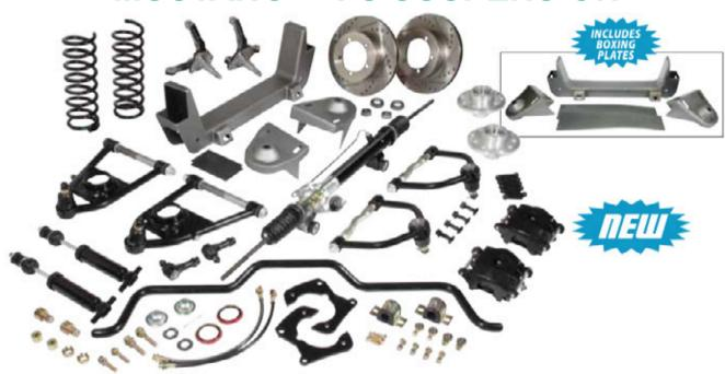
NOTE: Drilled and slotted rotors and black powder coated calipers pictured are extra, see upgrades
