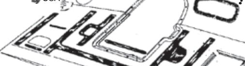
1. Start with sound dampener kit, self adhesive high density floor depression filler and sound dampener pads go in all indents on floor.
