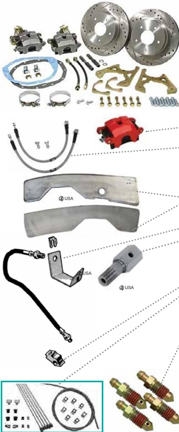
Brackets are not sold separately. Kit is set up for stock emergency brake cable. You must use a disc brake front and rear master cylinder & proportioning valve booster kit or similar set up.
