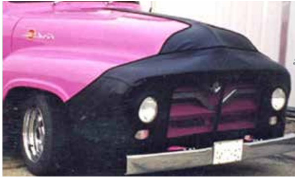
Bumper Mask is held on with bendable tabs
