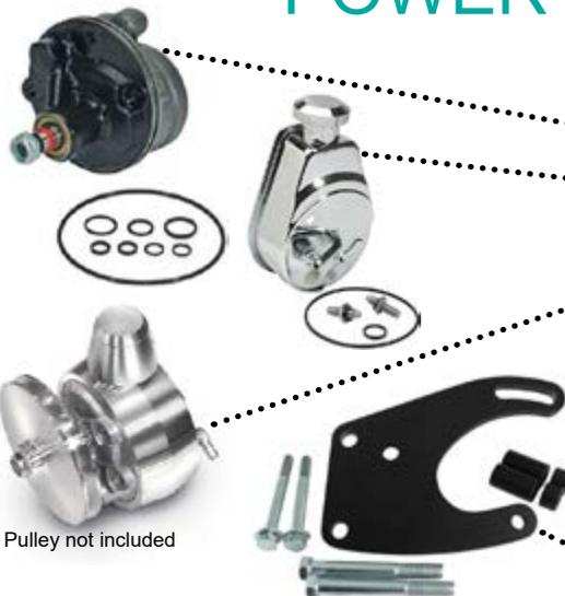
Brackets needs to match the engine, pumps need to mach the brackets and pulleys needs to mach the pump AND match your belt type
