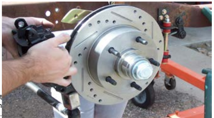
Mike installs the calipers on the front You know you're a true Mid-Fifty girl when you get excited over brake class.
