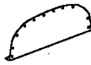
Locate both right and left sides, One hole needs drilled at rear. Remove plastic, shiny side goes out, toward wheel. This piece goes against bed side behind fender mounting flange. Use fender welt.
