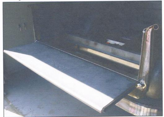
8. Once you are satisfied with the fitment in the closed and open position, fully weld all of the remaining holes and dress the welds for paint.
