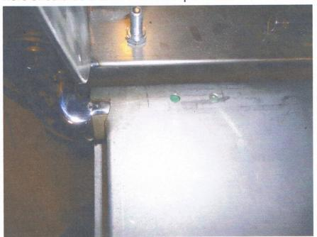
3. Slide the slotted piece into the bottom roll of the tailgate 1/4" to 1/2" and mount one hinge to the bed post.
