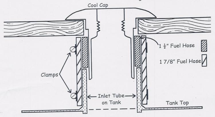
The 1  $\frac{1}{2}$ " hose will fit on the Cool Cap and fill the gap. Cut the 1 7/8" hose to fit from the tank up to the bottom of the wood.
