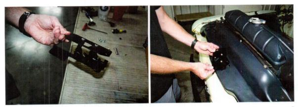
Step 5: Remove the old striker pin from the inside of your hood. This is done using a flat head screwdriver to hold the pin in place while you remove the jam nut on the back side of the inner hood panel. Once the nut is removed, the pin will screw out.
