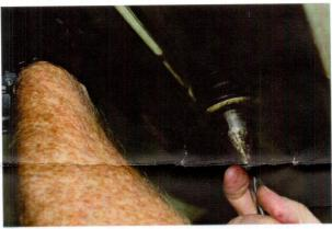
Step 6: Screw in your new Altman Easy Hood Latch striker assembly. You do not have to reattach the jam nut at this time, as you will be adjusting the pin to fine tune the closing of your hood. Thread the pin in until approximately ¼" of the threads are sticking through the welded nut on the inner hood panel. Make sure the nylon striker is lined up with the slot on your latch plate.
