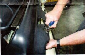
Step 3 : Prepare your new Altman Easy Hood Latch by loosely attaching the latch to the latch plate using the (2)  $\frac{1}{4}$ -20 X  $\frac{3}{4}$ " button head bolts and (2)  $\frac{1}{4}$ " hex nuts provided in your kit. These will be tightened later, but for now, having them loose will assist in installing the latch through the factory hole in the radiator support.
