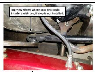
Steering stop limits the wheel's range of motion to prevent interference between the brake caliper and the axle on the passenger side of the dropped axle.
