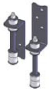
6. Using the sway bar end links as a template, mark and drill the 6 3/8" holes that will be used to mount the end link brackets.
