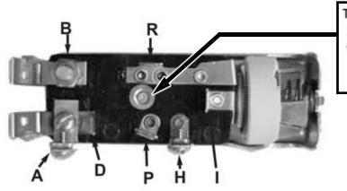
To release the shaft, push it as far into the switch as it will go then press and hold this button, and pull back on the shaft.
