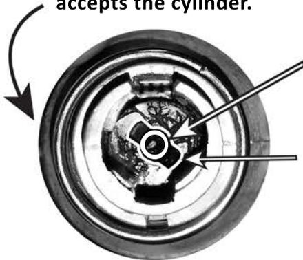
Looking down into the ignition cylinder you should see a small spring in the center of the slot in the bottom of the key way. There is a bit of white grease in this location, so it may be difficult to see. Make sure this spring stays inside the slot and is not sideways.
