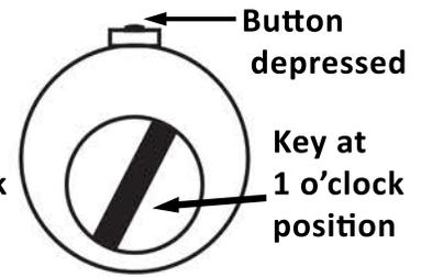
View of the ignition switch if you are looking down into the hole that accepts the cylinder.
