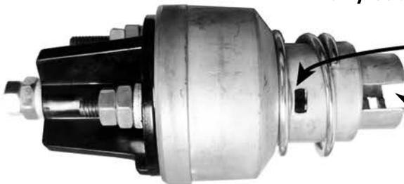
If the button does not come up high enough to poke through this hole, it's ok because this cylinder will be held in place by this slot. Once all of the pieces are installed in the dash, the bezel keeps the cylinder from slipping out of the switch.
