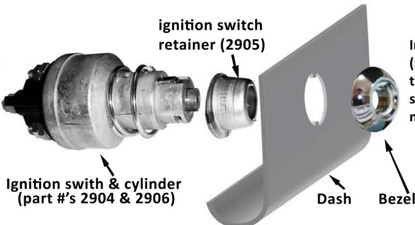
Installation into dash: Slip the retainer on the switch, (note the slot). Compress the spring, pushing the switch through the dash. Install the bezel by turning into the slot on the switch. Note some (mostly 1953) trucks may need the dash hole slightly enlarged.
