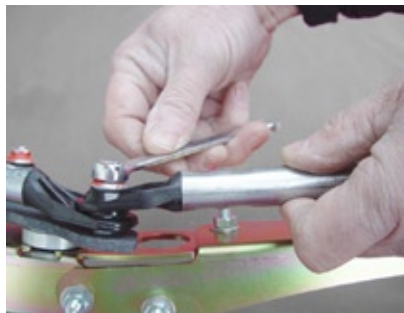
Photo 14. Slip the link ends of the Cross Link over the other link ends at "C" and "D".
