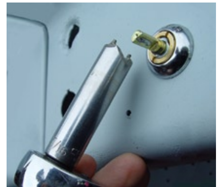
Photo 18. Add the chrome bezel and the switch nut. Use a pair of small screw drivers or make a special wrench from a 7/16: deep socket.
