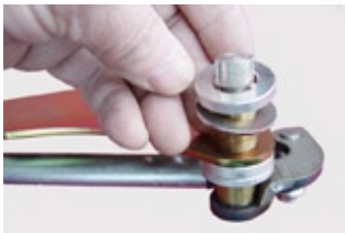
Photo 7. Place a stainless washer and one aluminum spacer onto each of the brass pivot shafts.
