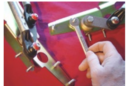
Photo 4. Use a 1/4" flat washer and a 1/4" hex nut to draw the flats of the bolt into the square hole.
