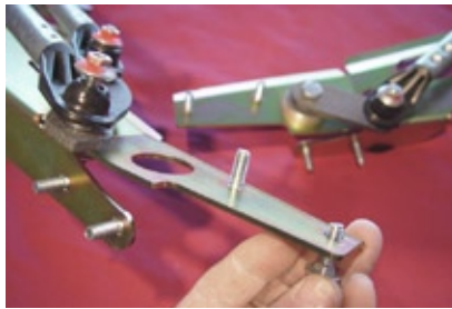
Photo 3. Add carriage bolts to the square holes in the Drive Unit & Follower Assy.
