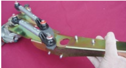
Photo 5. Attach the Bridge Spanner to the Drive Unit.
