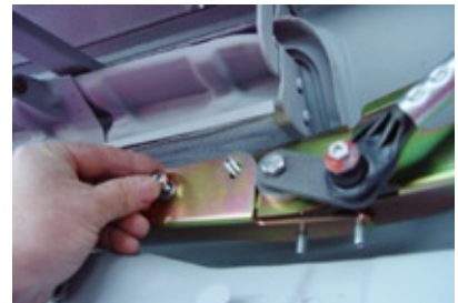
Photo 11. Add and tighten the nuts.
