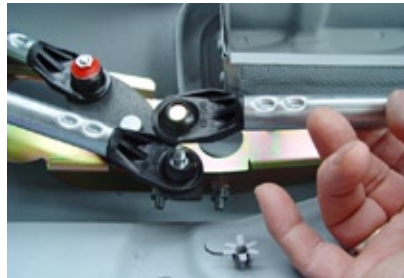
Photo 14. Slip the link ends of the Cross Link over the other link ends at "C" and "D".
