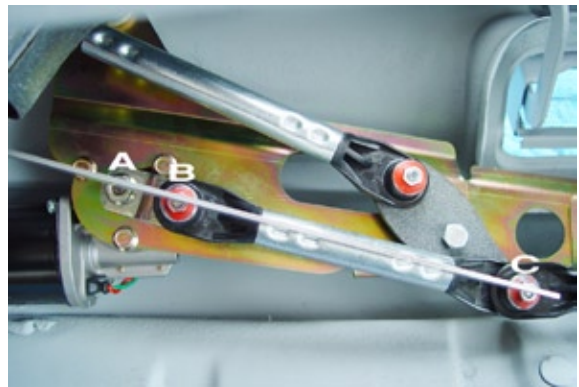
Photo 20. This is how the alignment looks when properly parking. Note that in the PARK position points A, B and C are in line along the straight edge.
