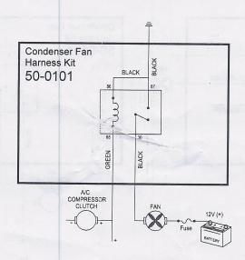
[part #24-0103] or Fan pressure switch [part #24-0104] is available from Old Air Products. For racing applications, where it is desired to manually engage the fans, a toggle switch may be mounted within the passenger compartment and connected to the 'Fan Switch' terminals.
