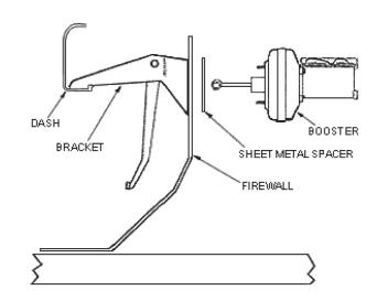
2. When all the holes are drilled, mount the booster and pedal assembly as shown to the firewall and dash. (Steering column drop mount holes)
