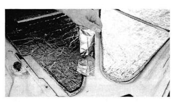
Install the seam tape around the edge of each of the insulation panels--overlapping the tape on to the rib of the hood.
