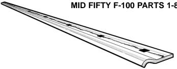
This cover piece does not have an angle. To keep it snug against the flange the last hole will need to be drilled through the bed side flange and bed wood.
