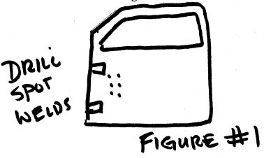
3. Cut door skin to allow access to inner door bracing. See picture # 2 you do not need to cut inner door skin above the hinge pocket. We recommend cutting only approx 8-10" below top hinge pocket.
